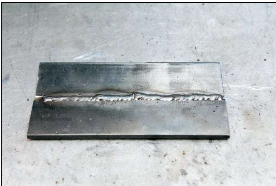
Figure 17. Completed weld runs
