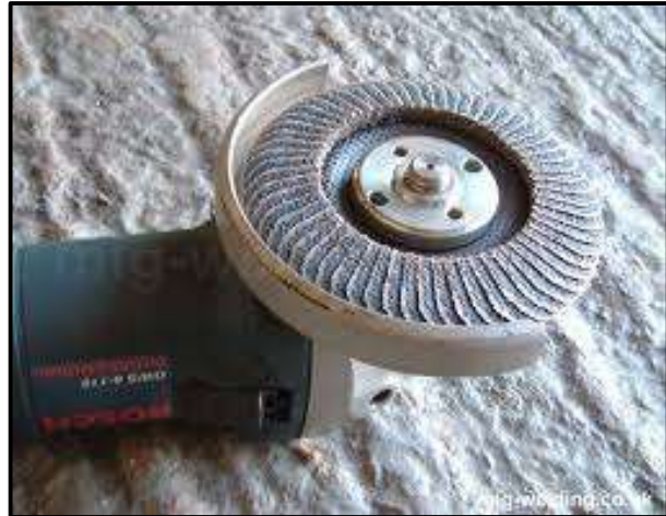
Figure 8: Flapper disc mounted on angle grinder
