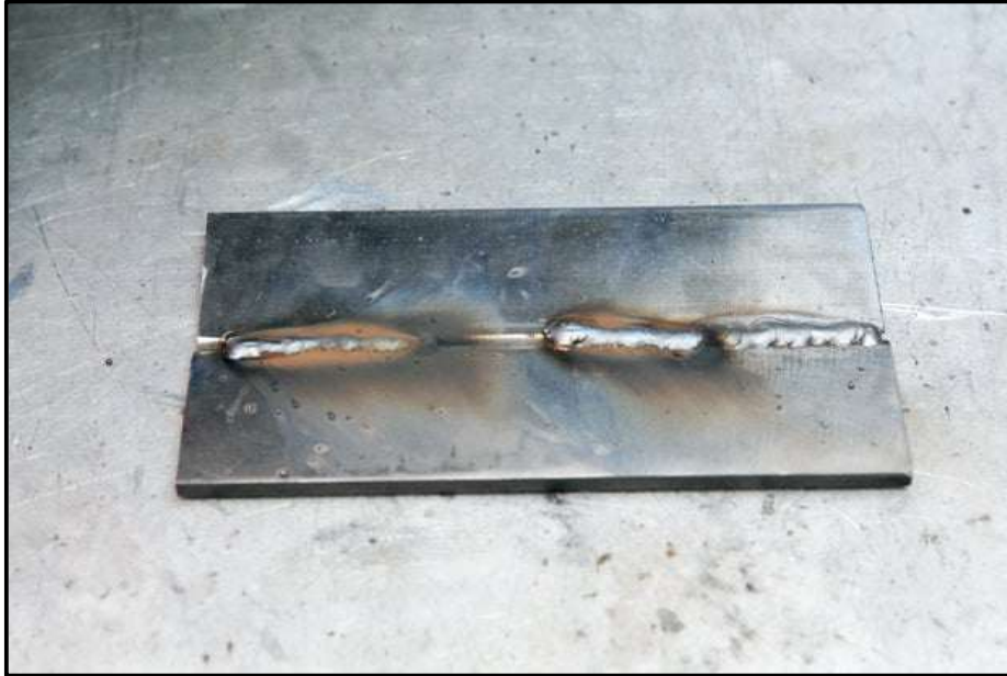
Figure 16: Start weld runs
